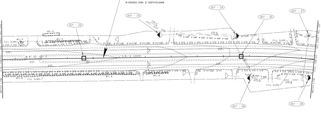
WHEN EXISTING PIPES ARE TO BE LEFT IN PLACE AND ABANDONED, THEY WILL BE BACKFILLED AND PLUGGED. NO MATERIAL FROM THIS PROCESS WILL BE ALLOWED TO LEAK INTO THE STREAMS.
